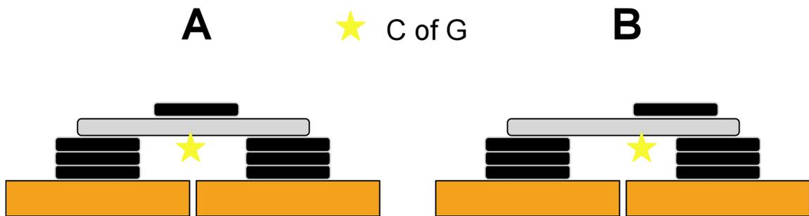
Fig. 2: Schematic representation of basic lab testing. Weights were stacked symmetrically (A) and asymmetrically (B) to test for reliability and sensitivity.
